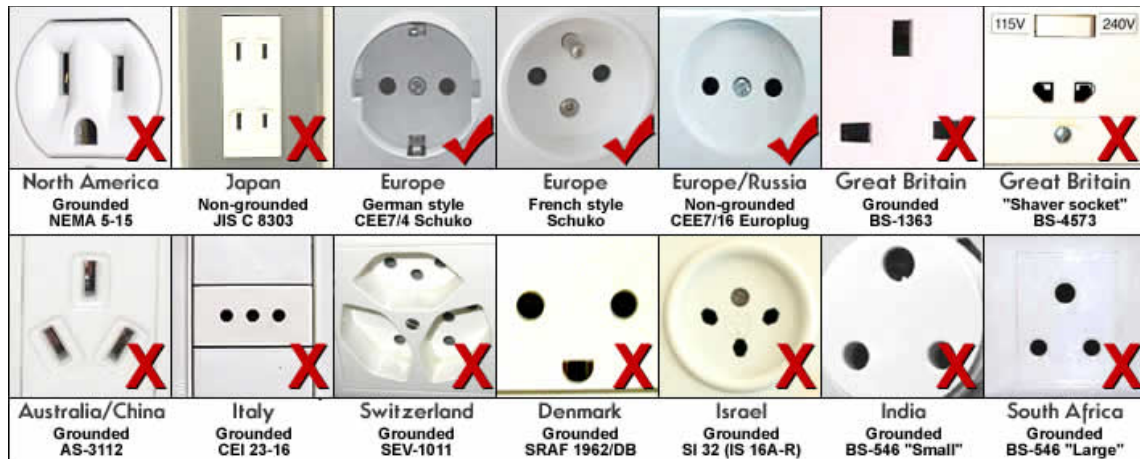
Photo 8: Plugs that work and don't work in Poland.
